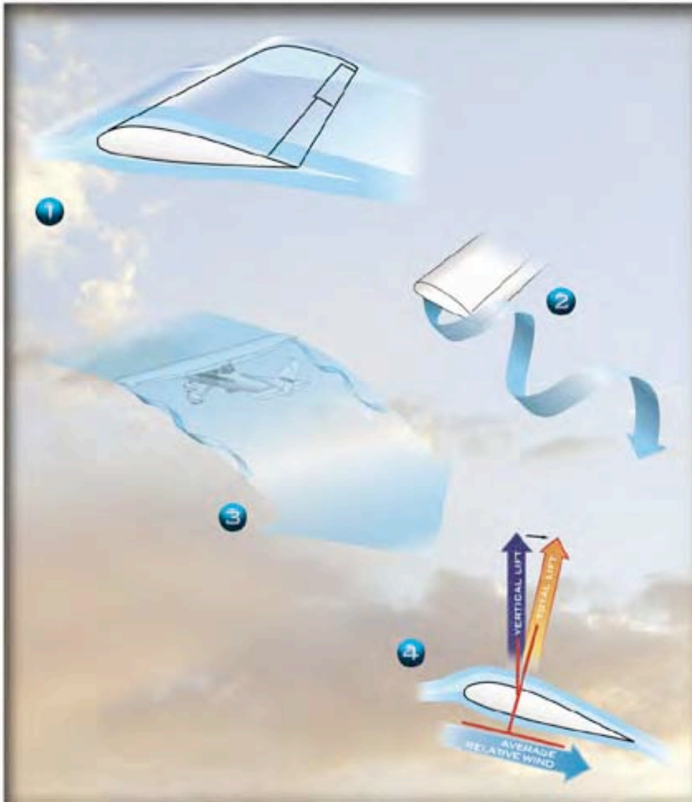
Figure 11 - Wingtip Vortices and Induced Drag
