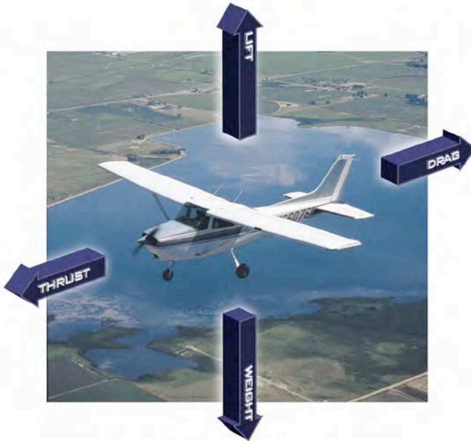
Figure 8 - In straight-and-level flight, all four forces are equal to each other
