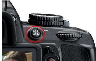
[Note: You can program the AF-L/AE-L button to 'AE lock (hold)' so that exposure locks when the button is pressed and remains locked until the button is pressed a second time (or the standby timer expires).]
