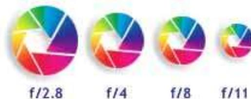
The maximum aperture of a lens is also called its lens speed. A lens with a large maximum aperture (f2.8) is called a "fast" lens because the large aperture allows you to use high (fast) shutter speeds and still receive sufficient exposure. The big advantage of these lenses fast lenses is that they are ideal for shooting moving subjects in low light conditions. Zoom lenses specify the maximum aperture at both the wide angle and telephoto ends (e.g. 28 - 200mm f3.5 - 6.3). A
