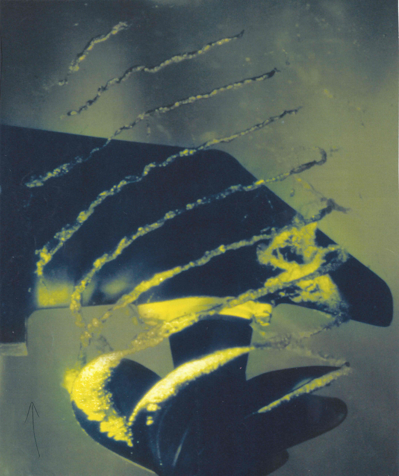
Cavitation on a modern ship propeller. This photograph was taken by Mark Dutweiler (PhD '01) in Caltech's Mechanical Engineering, Low Turbulence Water Tunnel. The flow is from right to left.
