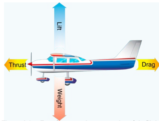
Figure 4-1. – Four forces acting on an aircraft in flight.
