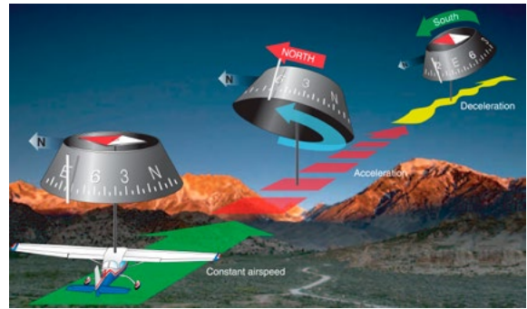
Figure 33-7. – The effects of acceleration error.
