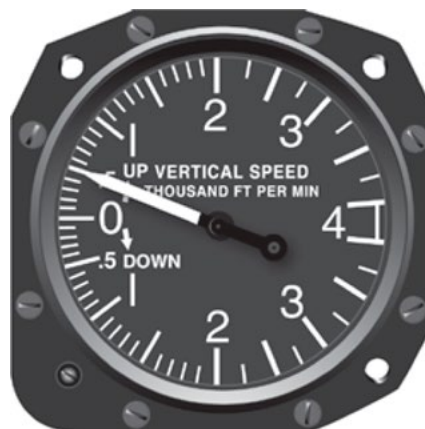
Figure 24-8. – Vertical speed indicator.
