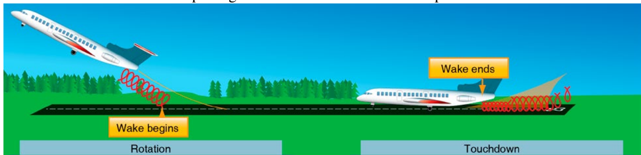
Figure 6-6. – Wake turbulence on takeoff and landing.
