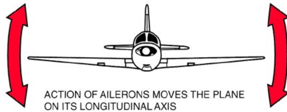
Figure 4-7. – Effects of the ailerons on the aircraft.
