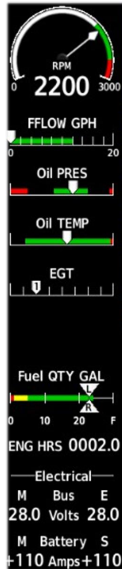
G1000NXi with GI-275 EIS Note the lack of vacuum system.
